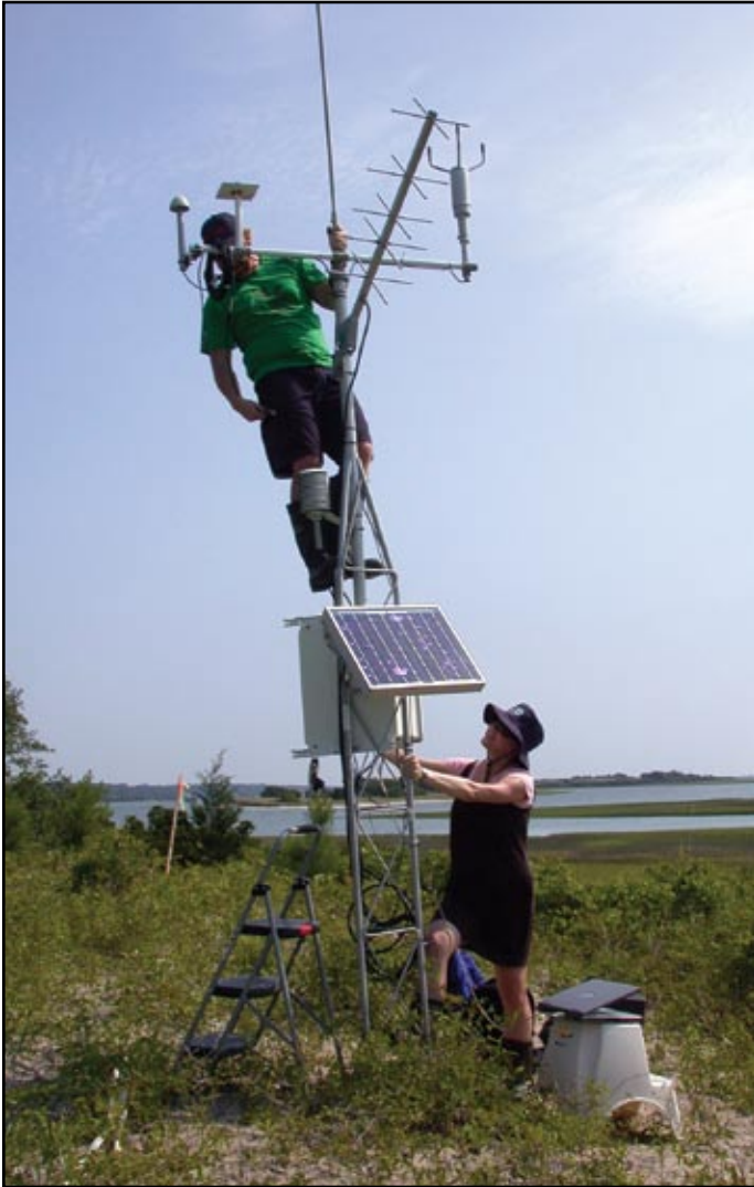
Figure 22. The North Carolina National Estuarine Research Reserve has recently upgraded monitoring stations to real time. In this photo Byron Toothman and Heather Wells are maintaining the meteorological station on Masonboro Island, NC. Photo NCNERR/Hope Sutton.
