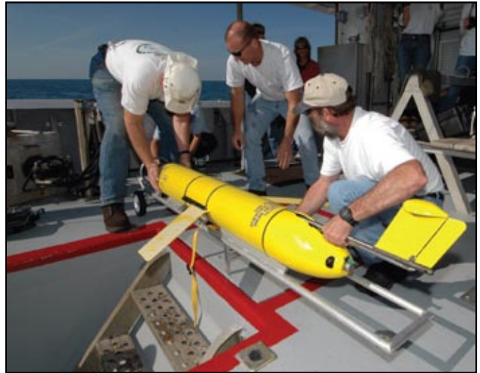
Figure 4. Autonomous underwater vehicles are deployed for up to 14 days and continuously collect data throughout the water column. For example, UNCW deployed the Slocum Glider, seen in the photo, before and after Hurricane Ophelia in 2005. The glider provided data showing changes in the water temperature, salinity, turbidity and chlorophyll a within Onslow Bay pre- and post-storm. Photo UNCW/Jamie Moncrief.
