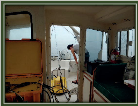
(Left): Erik Gudmunson prepares the CHIRP Sub-bottom Profiler for deployment on a calm day on the Albemarle Sound. (Right): Raw data from the CHIRP system on the Albemarle Sound showing paleochannels and shallowing water depths.
