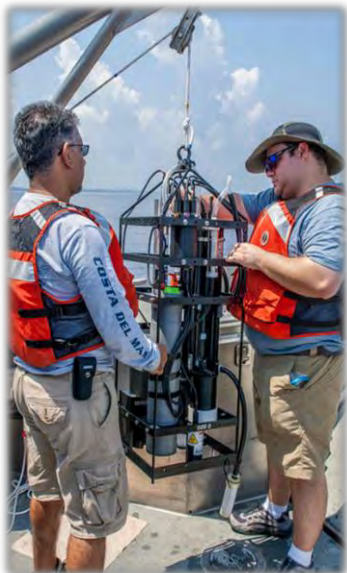
CRM PhD student Christopher Buonassissi (right) and ICSP research associate Dr. Ramon Lopez (left) prepare the Miller Lab's bio-optical profiling system.
